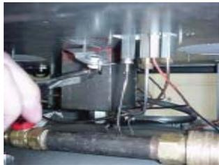
Tilt the blower onto its side and slide it past the controls. Position the blower onto the studs. The blower bracket contains slots that allow the blower to be positioned away from the intended gas supply hole. Secure the blower using the lock washers and wing nuts provided.
